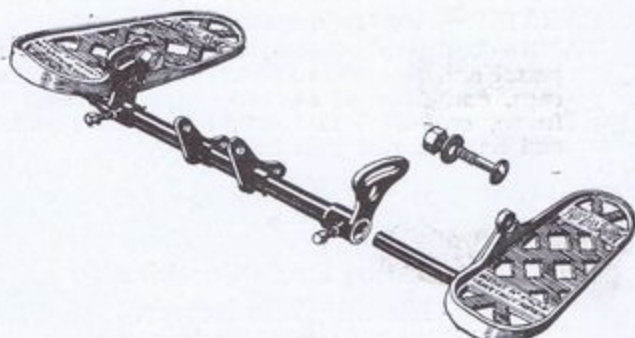
Royal Ruby adjustable footboards, made of aluminum, showing how easily they are detached, and also adjusted to the different positions required to suit the rider.
