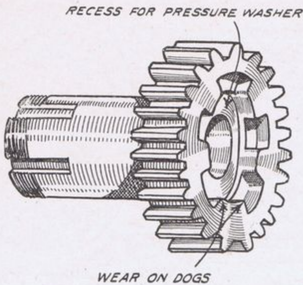
Fig. 47.—EXAMINING THE HIGH-GEAR PINION FOR WEAR ON DOGS.
