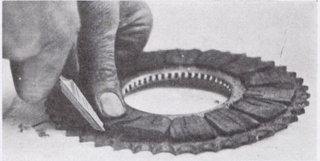
Fig. 38.—RECORKING THE CLUTCH PLATES.
