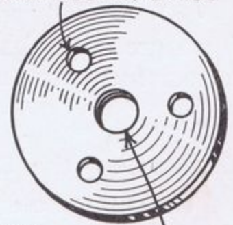
\frac{1}{2} " DIA. TAPPED SAME THREAD AS BOLT.
